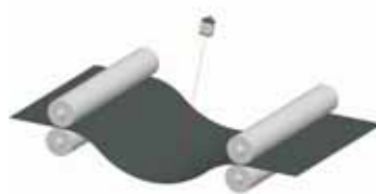
Web tension monitoring
